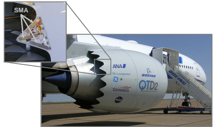
Figure 10. Boeing variable geometry chevron, flight testing [28].
