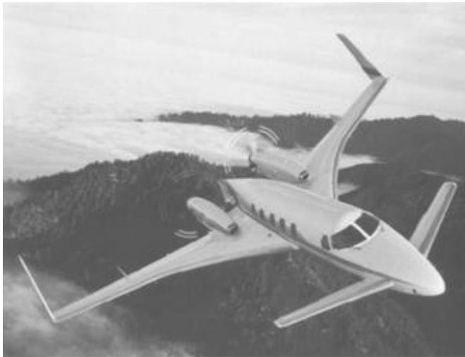
15.37 Beech Starship has a sandwich composite fuselage construction.
