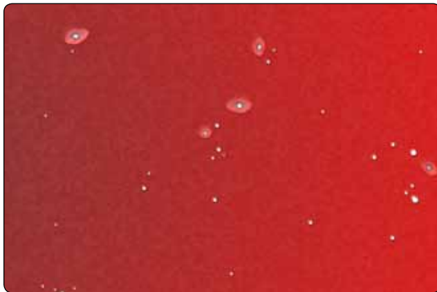
Figure 8-18. Example of fisheyes.
