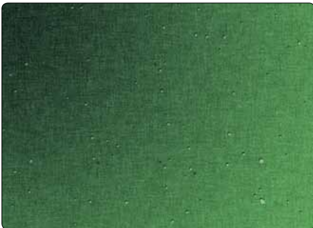
Figure 8-15. Example of pinholes.
