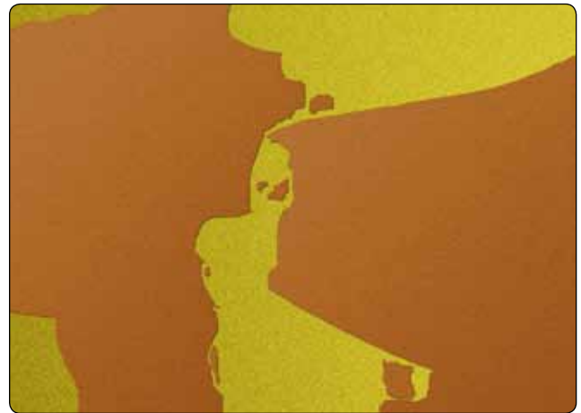
Figure 8-13. Example of poor adhesion.
