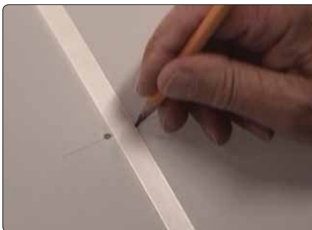
Figure 3-24. A premarked location for a lacing hole, which is punched through the fabric with a pencil.
