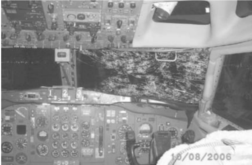
13.10 Hail damage to a cockpit window.
