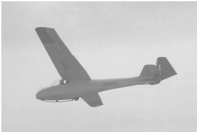
17.1 Application of wood in aircraft: glider made of spruce and ply. (photograph supplied courtesy of C. White)
