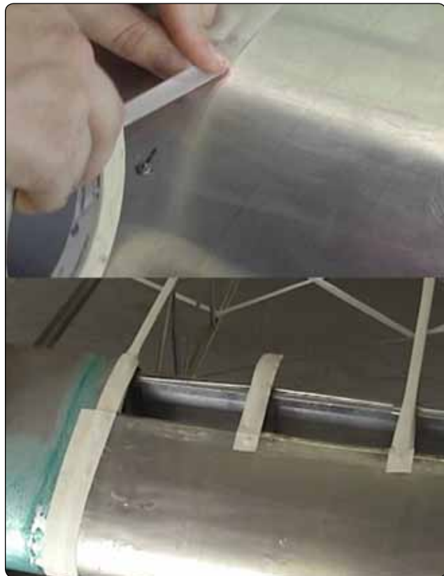
Figure 3-18. Anti-chafe tape is applied to all features that might cut or wear through the fabric.
