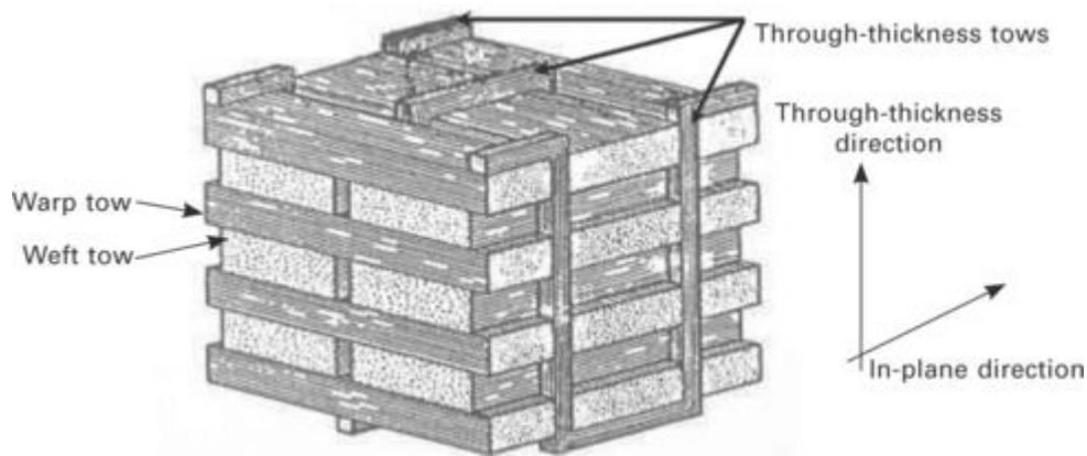
14.13 Three-dimensional fibre tow structure of fabrics.
