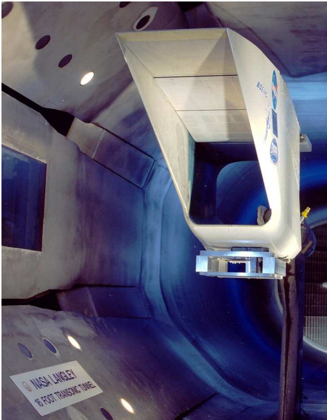
Figure 9. The SAMPSON F-15 inlet cowl as installed in the NASA Langley Transonic Wind Tunnel [20].
