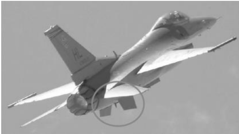
16.5 Al–SiC composites are used in the ventral fins (circled) and fuel access doors of the F-16 Fighting Falcon .
