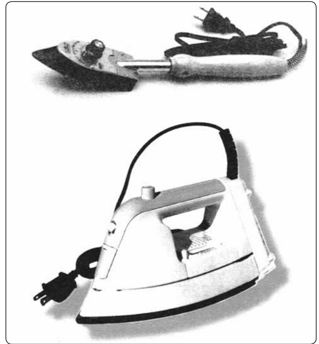
Figure 3-21. Irons used during the fabric covering process.
