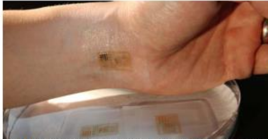
Fig. 3 Ultrathin path that mounts directly onto the skin with the flexibility and comfort of a temporary tattoo
